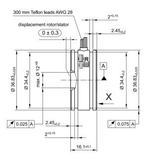
Inner diameter stator = 22.800 min. Outer diameter rotor = 22.325 max.
