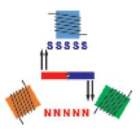
First, FOC applies to three phase Brushless Motors that are operating in sinusoidal mode. In sinusoidal commutation, all three wires are permanently energized with a sinusoidal current that is 120 degrees apart on each phase. This has the effect of creating a North/South magnetic field that rotates inside the motor cage. As shown in the figures below:
