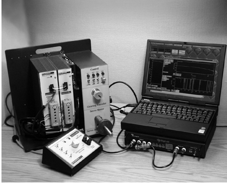
Kollmorgen ServoStar System (left) being measured by DSP Technologies SigLab, a Dynamic Signal Analyzer which uses a laptop computer Figure B
