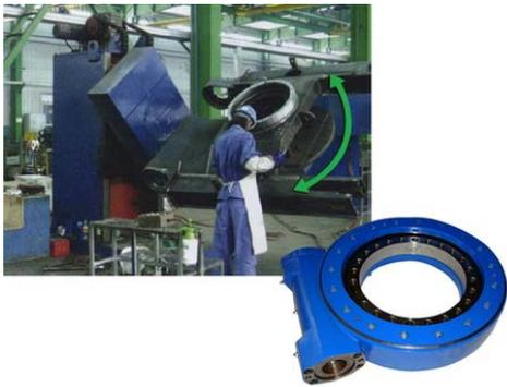
The rotation of welding machine is drove by SE series of slewing drives.
