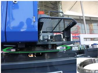
The R series of productions are fitted to slewing bearing as a new design in the field of work platform with cost-effective and reliable.
