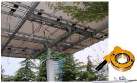
Controlling the solar components by horizontal and Elevation tracking, it will improve power generation efficiency with high return on investment. The slewing drives have been widely promoted in market of Europe, United States and China.
