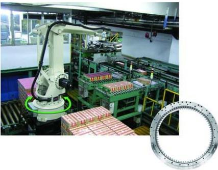
Slewing drives are widely applied on the rotation of joints.
