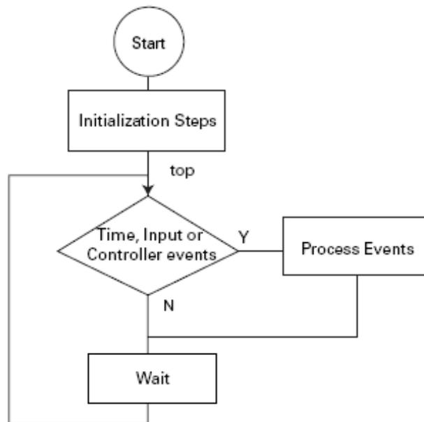
Often, some actions must be done only once when script starts running. This could be setting the controller in an initial configuration or computing constants that will then be used in the script's main execution loop.
