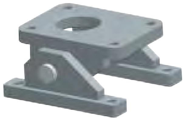
In order to allow worm gear screw jacks to carry out swiveling and tipping movements, the drive elements must be secured at two points and permitted to move. This can be done using a drag bearing arrangement and a head (IV) or coupling head, or by means of a swivel-lug configuration. The lateral force resulting from the swiveling motion should be minimized as much as possible by means of low-friction articulations.
