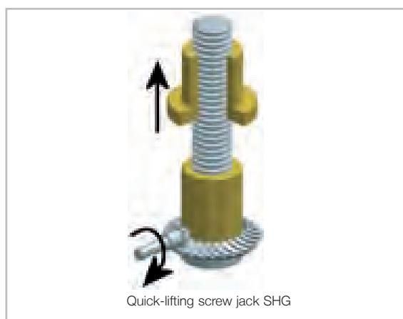
Drive is effected by the driving pinion acting on the bevel gear. Rotating movement is effected by the positive engagement of the screw in the bevel gear. Lifting movement is effected by the travelling nut anti-turn device fitted on site. The alignment of the bevel gear (Ro = wheel upside / Ru = wheel downside) determines the direction of rotation (see type 1).
