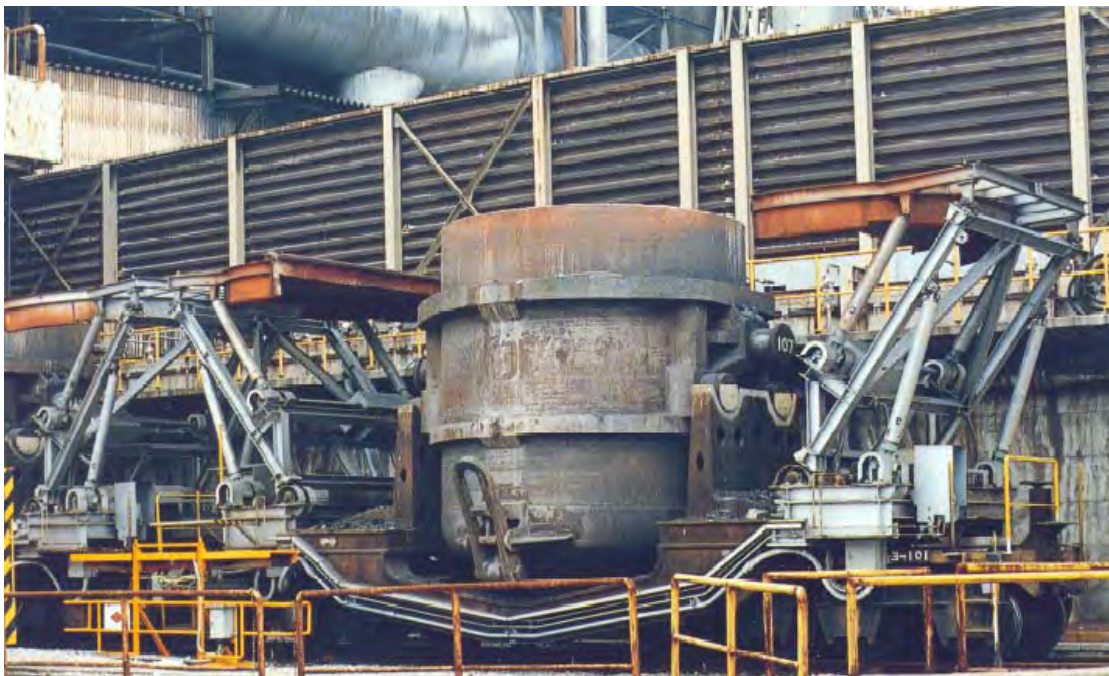
A pair of cylinders are parallel linked for operation. Eight sets of synchro-cylinders are used for one cart.
