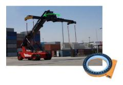
Slewing drive or bearing can be used in container crane.
