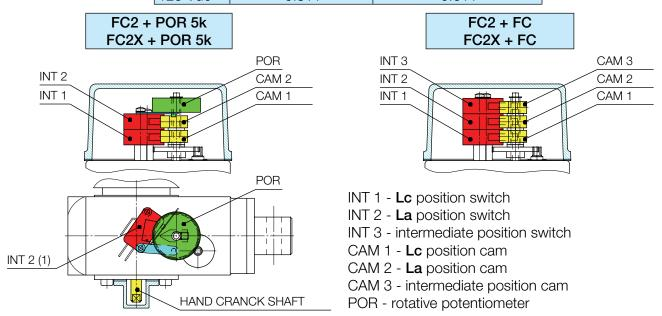
Lc = actuator retracted length, La = Lc + Stroke - actuator extended length
