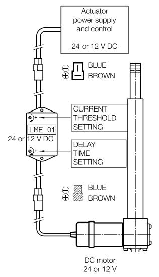
**LME 01** is an electronic device that protects DC motors against current overloads due to a persistent dynamic overload applied on the actuator.
