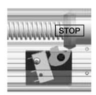
Standard switches have silver-plated contacts, max. current 12 A with resistive load - 6 A with inductive load. Switches with gold-plated contacts, very low contact resistance for low working voltage (if connected to PLC or PC), max. current 0.1 A, available on request.
