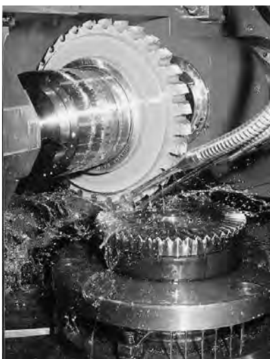
CNC machining of a PowerTRUE right-angle gear
