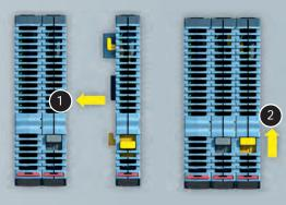
The positive "click-to-lock" mechanism firmly clamps Flexslice modules to each other to form a Flexslice station. Simply push each module together and slide the quick release locks into position.
