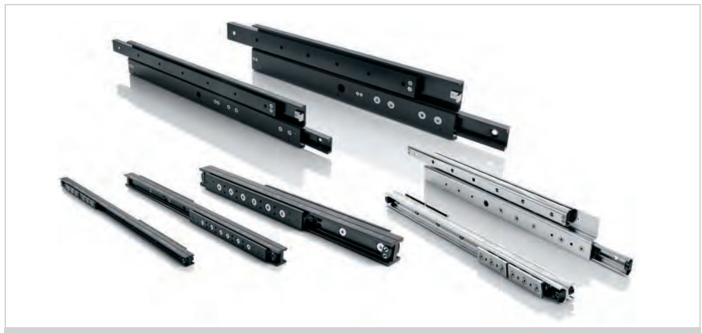
Fig. 6 - The Telerace family from Rollon includes 3 series of telescopic rails: TLR-TLQ high performance steel rails with double row ball bearings; TLN-TQN rails in profiled sheet with ball bearings; TLAX-TQX like previous series but in stainless steel.
