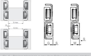
Fig. 5 - Telerace telescopic guides from Rollon can manage misalignment of the assembly surfaces thanks to axial floating rollers.
