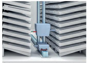
Fig. 3 - In automated warehouses, telescopic rails extract parts from the shelf and load them onto the carriage, or vice versa.
