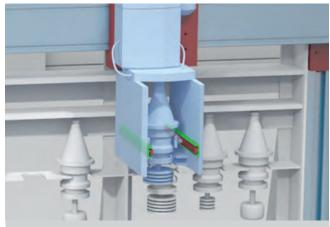
Fig. 1 - Tool changer: a bilateral stroke enables the telescopic rail to extract the tool and position it in CNC machine.
