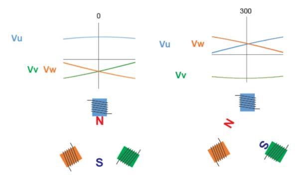
If a magnet is placed on a rotor inside this cage, its North and South poles will be pulled towards the South and North poles of the rotating field. Assuming for a moment that the magnetic field rotation is paused, we can see the effect of the pull on the magnet at different angular position relative to the rotating field.
