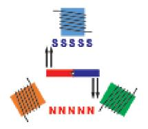
First, FOC applies to three phase Brushless Motors that are operating in sinusoidal mode. In sinusoidal commutation, all three wires are permanently energized with a sinusoidal current that is 120 degrees apart on each phase. This has the effect of creating a North/South magnetic field that rotates inside the motor cage. As shown in the figures below:
