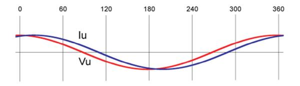
Back to our example, if the current follows the current as this chart shows, the magnetic field will not be 90 degrees apart from our rotor anymore but around 70 degrees. The rotor will not be pulled optimally. Part of the field will pull the rotor perpendicularly, thus creating torque, another part of the field will pull the rotor outwards.
