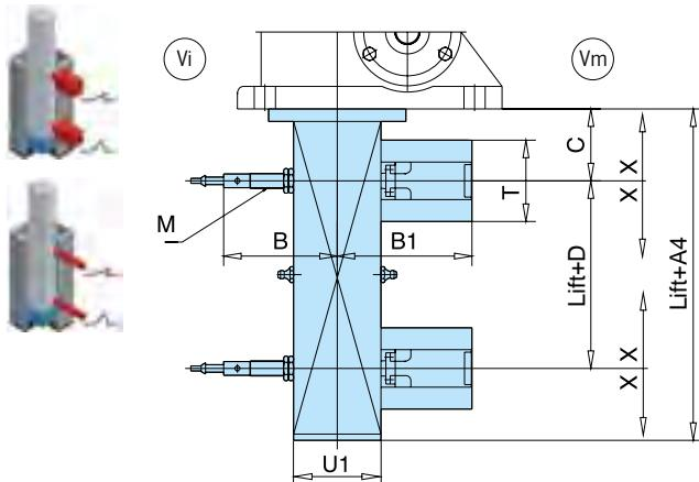
All sizes are prepared for mechanical (Vm) and inductive (Vi) operating limit switches.
