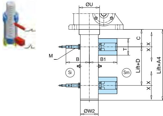
All sizes are prepared for mechanical (Sm) and inductive (Si) operating limit switches. Limit switches are not included in
