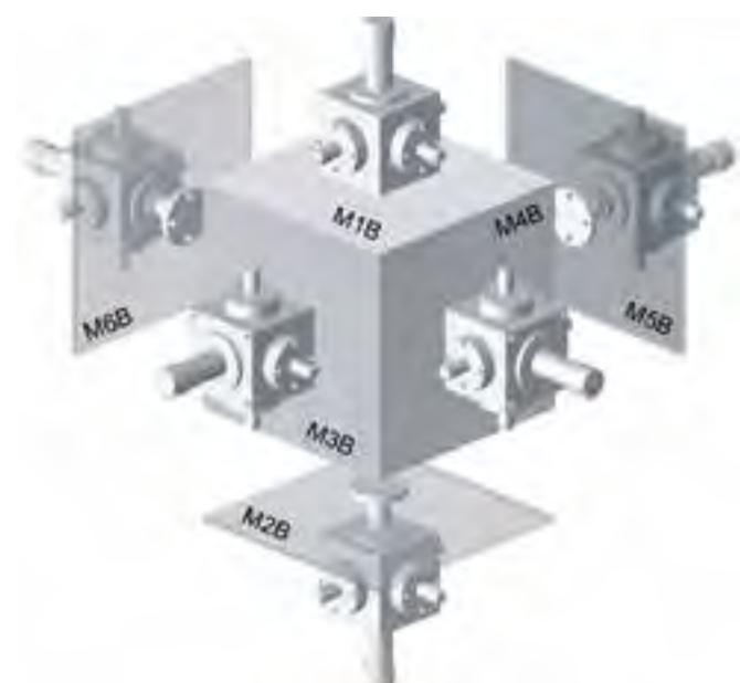
Shaft layout/Position of the oil fittings (b/c/d) - View from screw side
