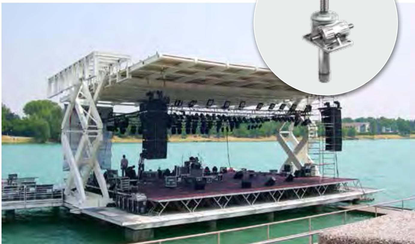
Optimized worm gear screw jacks from Pfaff-silberblau reliably and, above all, safely raise and lower the roof of Milan's lake stage.
