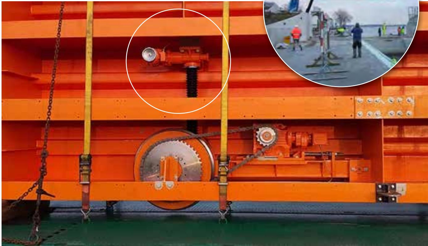
Fig. 1: Close-up view of the gate with the SHE 25 from Pfaff-silberblau for adjusting the travel wheel (copyright: ARGE HPI/hpl Greifswald)
