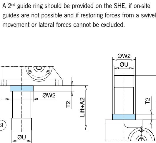
A 2<sup>nd</sup> guide ring should be provided on the SHE, if on-site guides are not possible and if restoring forces from a swivel movement or lateral forces cannot be excluded.
