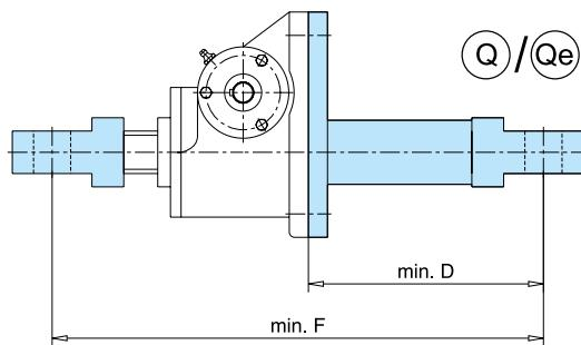
screw ends or an articulated head. The bending moment resulting from the swiveling motion should be minimized as much as possible by means of low-friction articulations.
