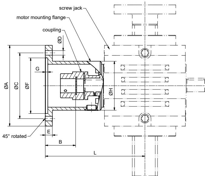
Dimensions motor mounting flanges: HSE range
