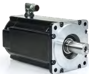
AKM2G-6x Flange: 142 mm Power: 1.56 - 7.79 kW Max Speed: 6000 RPM Stacks: 4
