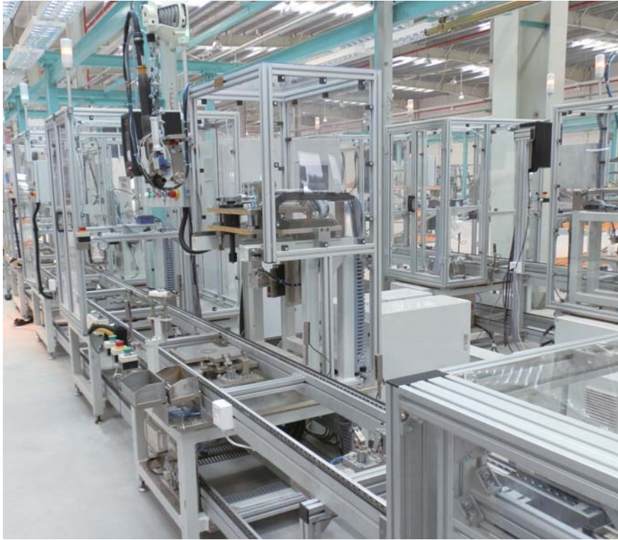
Machine guard frame for conveying equipment 输送设备防护框架
