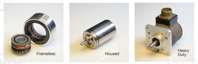
**Frameless Brushless Resolvers** generate speed and position data for aerospace & defense applications as well as commutating brushless servo motors. The frameless construction simplifies mounting mechanics because the rotor mounts directly onto the motor shaft and the stator housing mounts directly onto the motor end bell.
