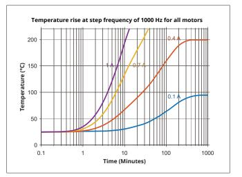
Use of the embedded temperature sensor is essential for motor protection. Irreversible damage of the motor windings will occur if the temperature exceeds the stated maximum operating temperature.
