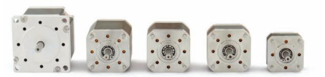
The model D motors are two phase hybrid stepper motors, available in a range of standard sizes and torque ratings. Standard motors provide 200 full steps per revolution, are suitable for use below 1x10<sup>-10</sup> mbar and working temperatures between -65 °C to +190 °C. Extended low temperature range (-196 °C) versions, radiation hard versions (1 x 10<sup>6</sup> Gy), shaft modifications and hybrid bearings are all available options.
