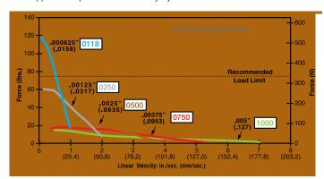
NOTE: All chopper drive curves were created with a 5 volt motor and a 40 volt power supply. Ramping can increase the performance of a motor either by increasing the top speed or getting a heavier load accelerated up to speed faster. Also, deceleration can be used to stop the motor without overshoot.
