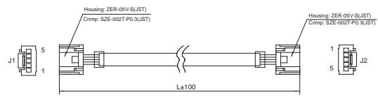
◇ RS-232 Communication Cable(P/S/Q Type)(TSM23/24/34)
