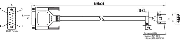
◇ Ethernet Daisy Chain Communication Cable (Q/IP Type) (TSM34 only)
