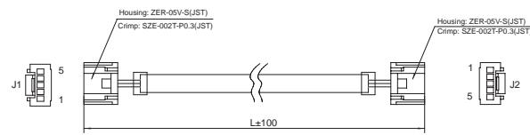
◇ RS-232 Communication Cable(C Type)(TSM17/23/24/34)
