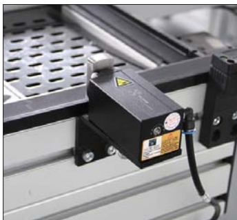
BU.PN.02/A-60 installed at the joint of the conveyor. It is used to buffer and stop the pallet infeeding or outfeeding from the main conveyor. BU.PN.02/A-60安装于线体对接处，用于缓冲并挡停移入移出主线体的托盘
