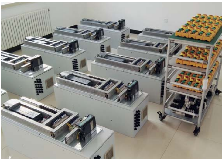
Electrical Control Cabinet 电控柜
