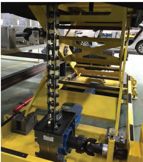
Lifting platform for automotive industry : HD Lift 60S lifting chain.
