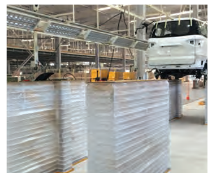
Lifting system for automotive industry: ChainLift with bellow cover
