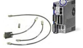
The CAN Termination connector is required for bus termination of the last AKD connected to the CAN bus. For connecting an AKD to a CAN device with SubD9 connector the CAN RJ12-SubD9 adapter can be used.
