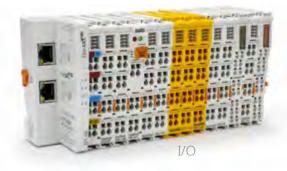
Kollmorgen Automation Suite<sup>™</sup> includes an array of I/O options for applications that need more I/O than can be provided by the onboard I/O of the drives or for applications that need specialized functionality such as thermocouple management through I/O. The DIN rail mount IP20 terminals simply slide together and connect to the system's EtherCAT<sup>®</sup> bus where they are autorecognized for easy configuration.
