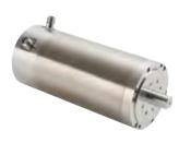
These brushless servo motors incorporate pressure compensation technology to allow underwater operation up to 20,000 ft while withstanding extreme environments. They feature stainless steel and aluminum nickel bronze housings. All shafts are stainless steel and sealed with an externally serviceable O-ring seal.
