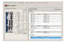
Embedded wiring diagrams and oneclick I/O variable mapping makes drive integration easy.
