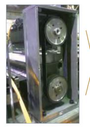
Press feed machine built with a conventional servo motor, gearbox, belt and pulleys.
