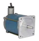
The explosion-proof MX Series provides hazardous-duty stepper motors suitable for use in Class 1, Division 1, Group D locations. They are available in NEMA 34 and 42 frame sizes (90 and 110 mm), and provide minimum holding torques from 1.27 to 9.82 N-m (180 to 1390 oz-in).
