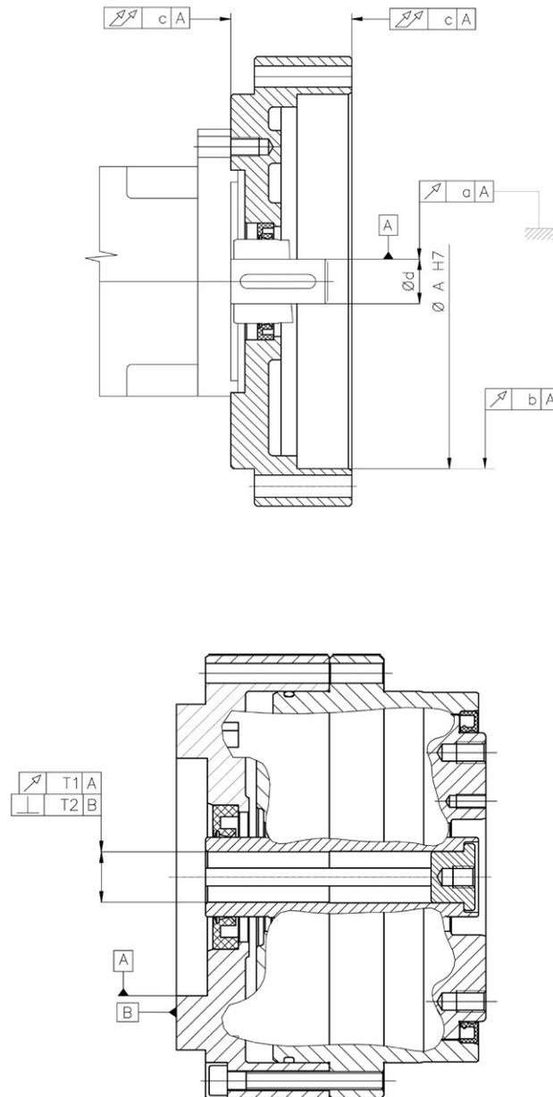
Fig. 5.2.4a: Geometric deviations for connection of the E series TwinSpin® high precision reduction gear flange or of the TwinSpin® E series reduction gear with a motor
