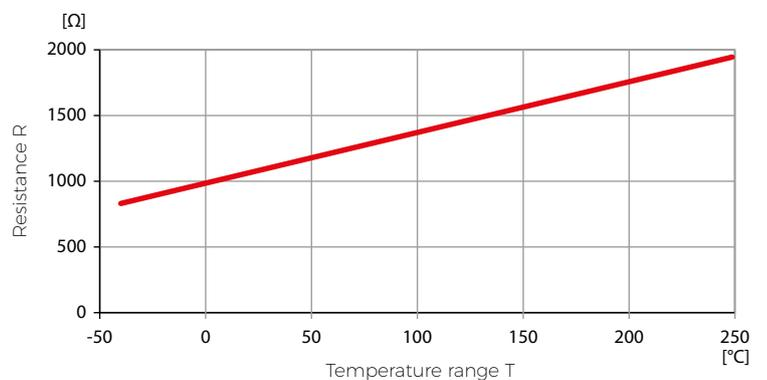
Fig. 8.5.k: Resistance / Temperature PT 1000
