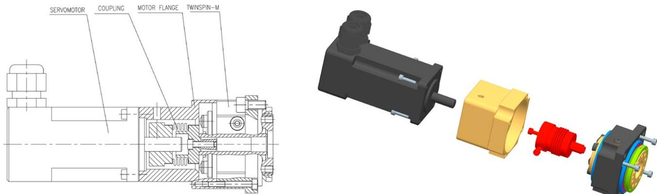
Fig. 5.4.1b: Shaft connection with flexible coupling
