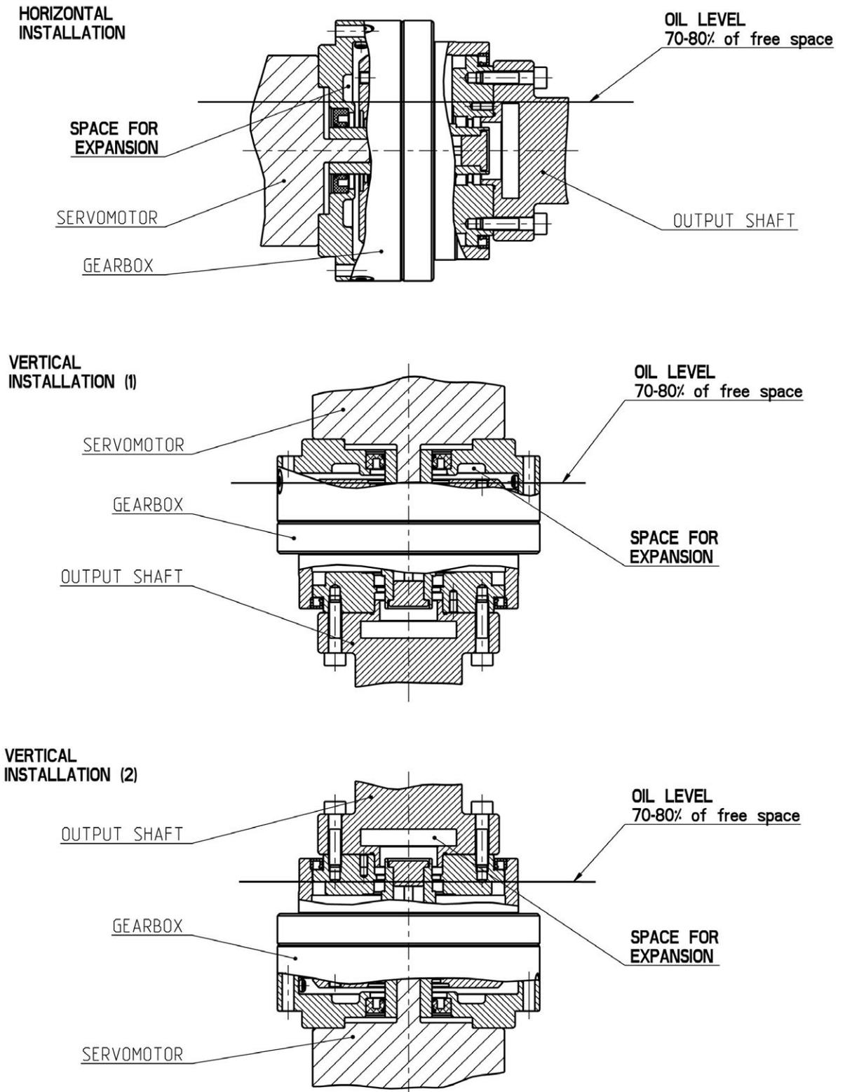
Fig. 5.5a: Lubricant levels in horizontal and vertical positions
