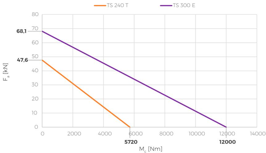
Fig. 3.5: Relation between the moment and axial force
